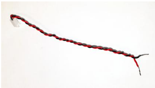
Figure 9: Two-pin Molex to bare wires for tests and LEDs for digital outputs
