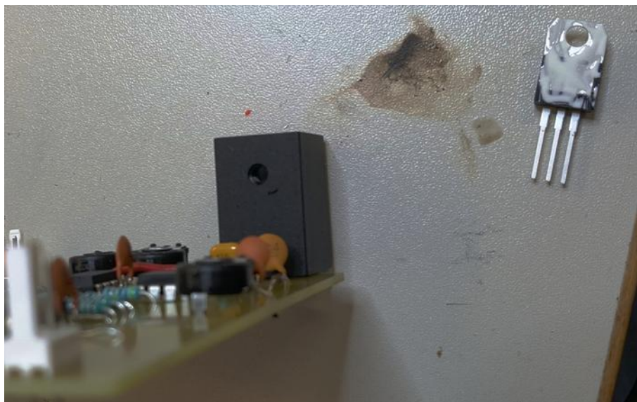
Figure 5: Soldered heatsink and thermal paste pre-applied to TO-220 device
