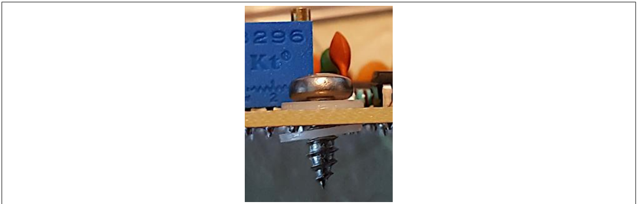
Figure 7: Adding washers to attempt to compensate for longer screws
