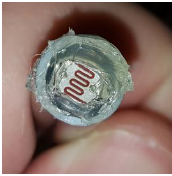
Figure 8: LDR mounted in plastic tube from ballpoint pen
