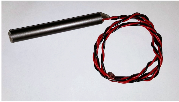
Figure 8: LDR mounted in plastic tube from ballpoint pen
